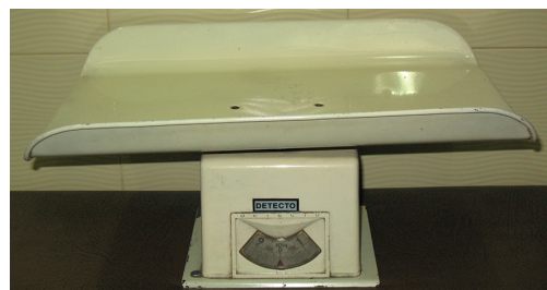
Figure 2.3 : Pan-type infant-weighing scale
