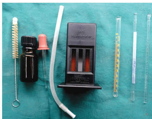
Fig. 7.2: Reagents and equipment for Sahli's method
