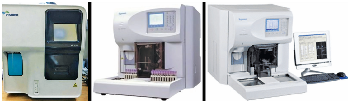
Fig. 15.2: 3-part, 5-part and 7-part haematology analysers
