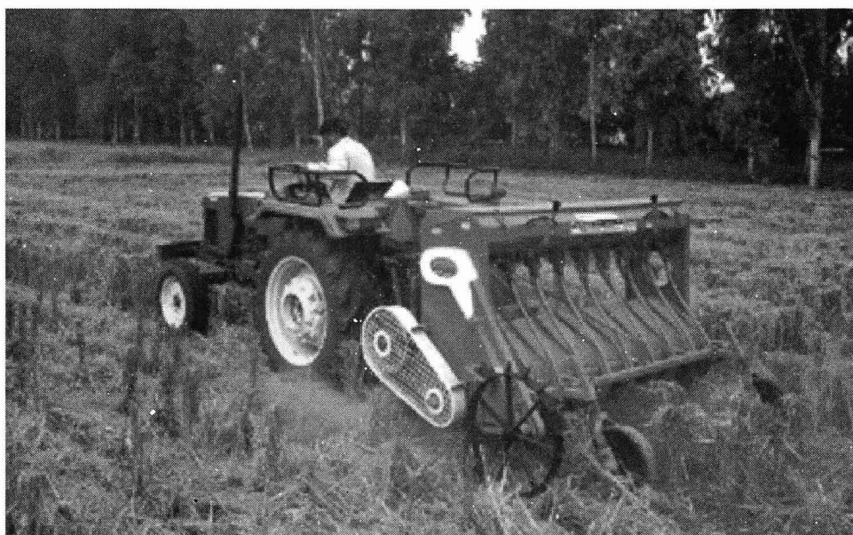
Fig. 2.6: Sowing of wheat with Happy Seeder in standing stubbles of paddy (see Colour Plate 2)
