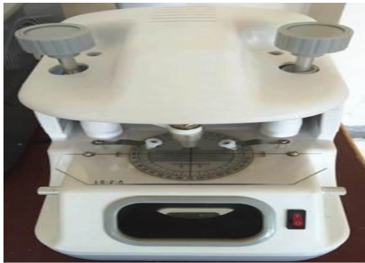
Fig. 16.2: Automated axis marking machine
