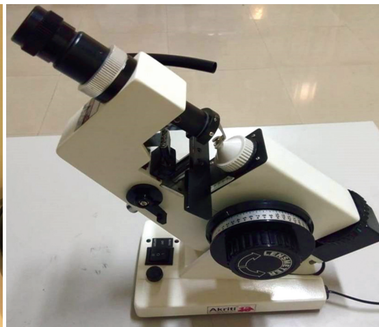
Fig. 6.1: An example of manual operated lensometer Fig. 6.2: An example of an automated lensometer
