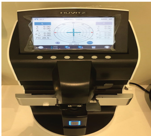
Fig. 6.1: An example of manual operated lensometer Fig. 6.2: An example of an automated lensometer
