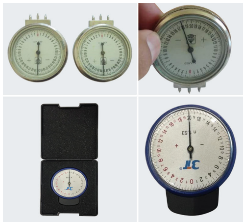
Fig. 6.3: An example of geneva lens measure (power and thickness of unknown lens)
