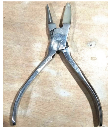
Fig. 11.18: Hand friendly slim nose pad arm adjusting plier
