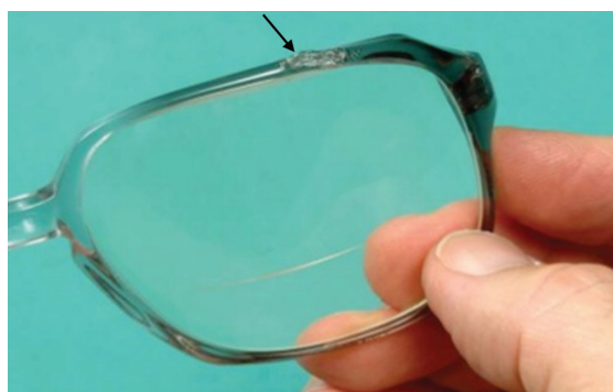
Fig. 13.1: Bubbling of the plastic upper rim due to overheating
