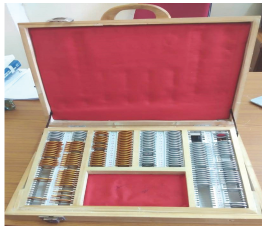
Fig. 6.4: An example of trial box (neutralization of unknown lens)
