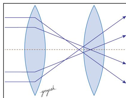
Fig. 1.4: Spherical aberration.
