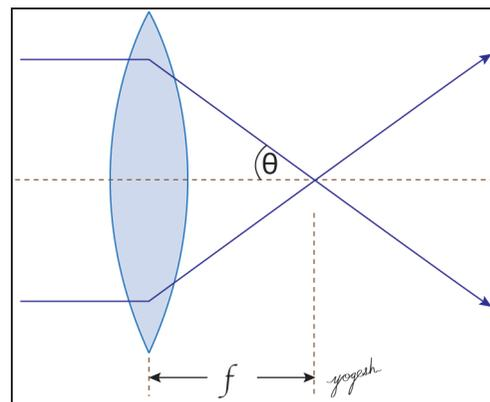
Fig. 1.2: Focal length (f) and numerical aperture ( $\theta$ ).
