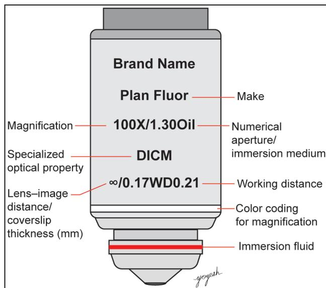
Fig. 1.5: Markings on objective lens.
