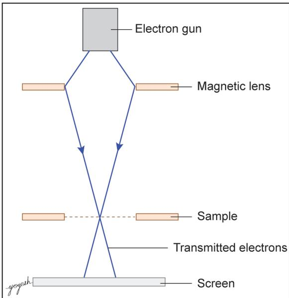
**Fig. 1.7:** Working principle of a transmission electron microscope.
