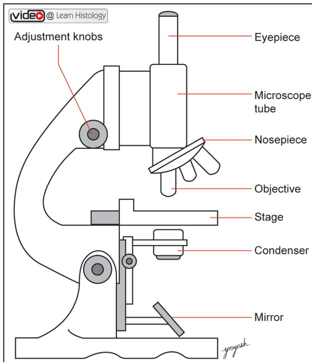
Fig. 1.1: Practice figure: Parts of microscope.
