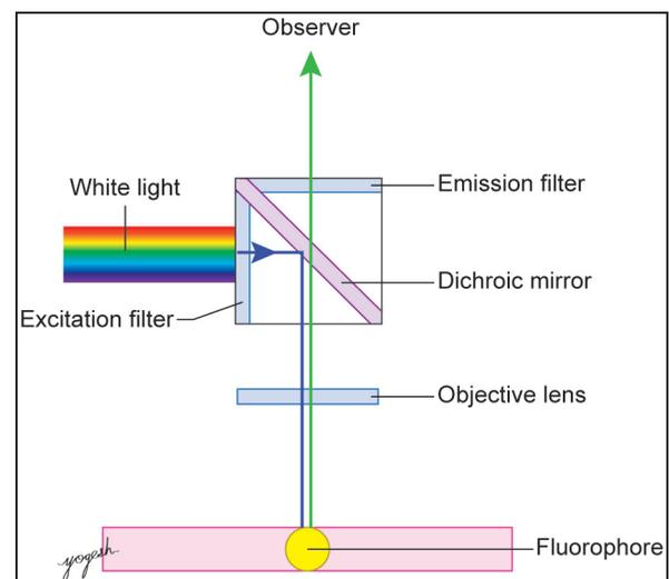
Fig. 1.6: Light path for fluorescence microscopy.
