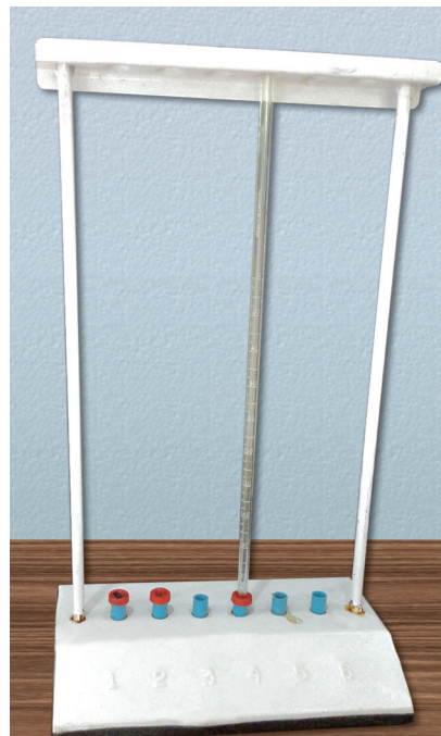
Fig. 1.22b: Westergren's pipette with stand
