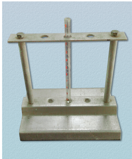
Fig. 1.21b Wintrobe's tube with stand
