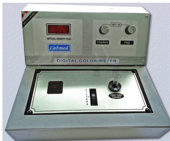
Fig. 1.13: Photocolourimeter for haemoglobin estimation by cyanmethaemoglobin method
