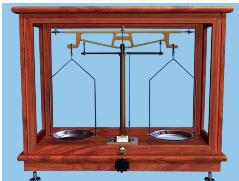
Fig. 1.1: Physical balance in closed compartment
