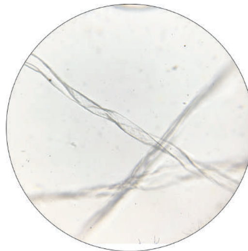
Fig. 1.1.11: Cotton fibers (a) low power (10 \times ) and (b) high power (40 \times ) of microscope.
