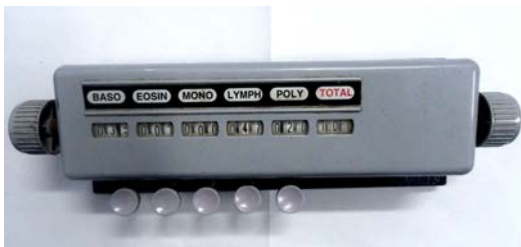
Fig. 2.11: DLC counter (manual) for differential leucocyte count (DLC)
