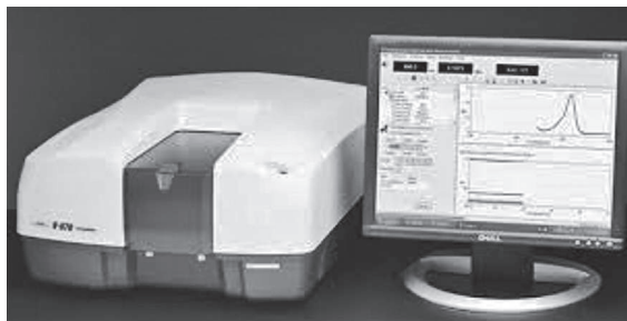
Fig. 1.1: UV spectroscopy instrument
